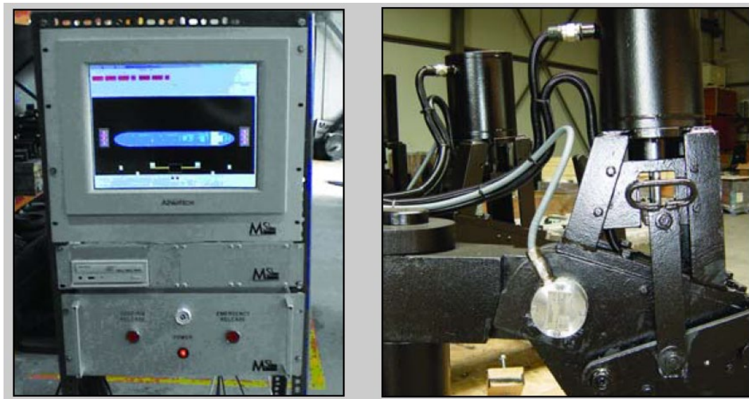
Figure 5 – Computer and Load Cell
